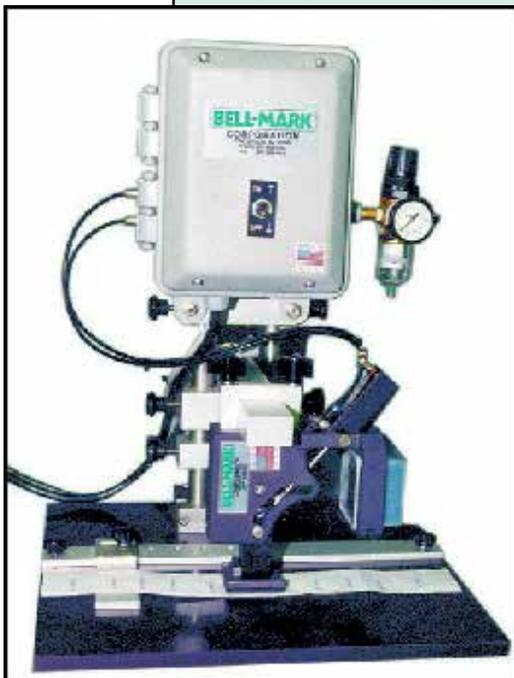
The US-4300 Coder is an air operated reciprocating coding system, foot activated by the operator to print on both absorbent and nonabsorbent surfaces.
